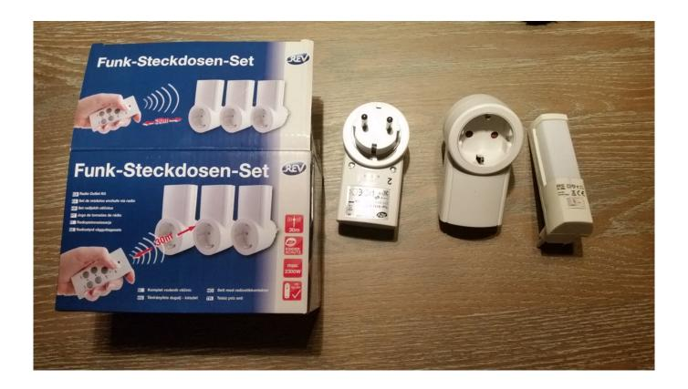
After recording the signals for about 30 seconds, I ran the following command to send the signals recorded by the HackRF One device to the RF outlet. After a short while, I experienced the RF outlet-connected light turning on and the signal being easily repeated (REPLAY) with HackRF One.
