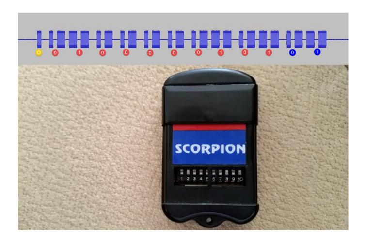
From now on, it was just a matter of modulating the data with ASK and sending it to the garage door, whether with Arduino or Raspberry Pi. Of course, for this I had to first get an RF transmitter and receiver kit, setting aside the 4\$. (For those who can't be bothered to do this type of security research, you can avoid all this hassle by spending 330\$ on a HackRF One kit like I did. By the way, you can also access free Software Defined Radio (SDR) and HackRF One training here.)
